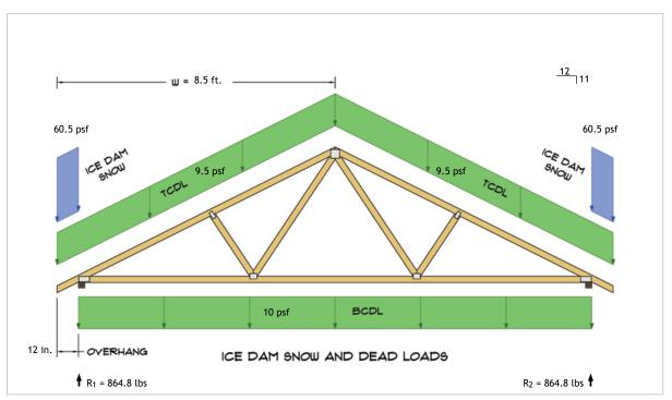
$R_1 = D + S = 622.9 \text{ lbs} + 241.9 \text{ lbs}$  $R_2 = D + S = 622.9 \text{ lbs} + 241.9 \text{ lbs}$
