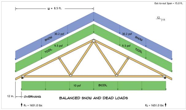
$R_1 = D + S = 622.9 \text{ lbs} + 1028.2 \text{ lbs}$  $R_2 = D + S = 622.9 \text{ lbs} + 1028.2 \text{ lbs}$
