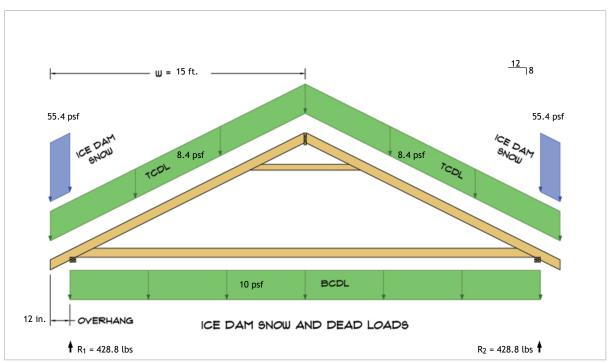
$R_1 = D + S = 354.9 \text{ lbs} + 73.9 \text{ lbs}$  $R_2 = D + S = 354.9 \text{ lbs} + 73.9 \text{ lbs}$
