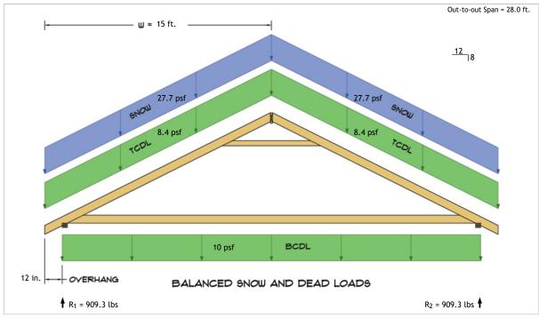
$R_1 = D + S = 354.9 \text{ lbs} + 554.4 \text{ lbs}$  $R_2 = D + S = 354.9 \text{ lbs} + 554.4 \text{ lbs}$
