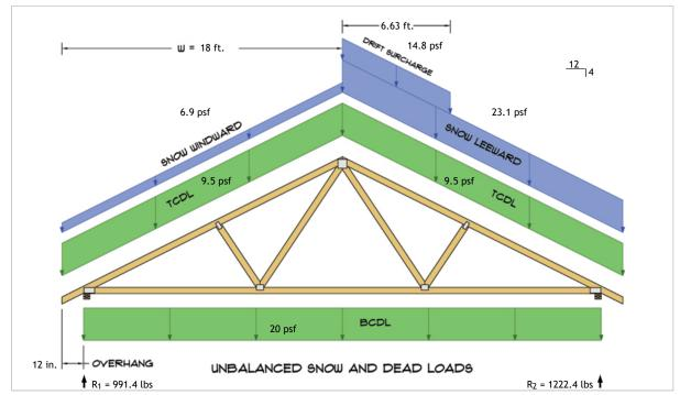
$R_1 = D + S = 681.0 \text{ lbs} + 310.4 \text{ lbs}$  $R_2 = D + S = 681.0 \text{ lbs} + 541.4 \text{ lbs}$
