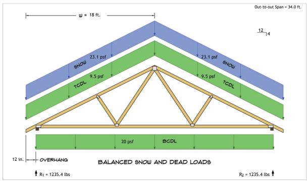
$\begin{aligned} R_1 &= D + S = 681.0 \text{ lbs} + 554.4 \text{ lbs} \\ R_2 &= D + S = 681.0 \text{ lbs} + 554.4 \text{ lbs} \end{aligned}$
