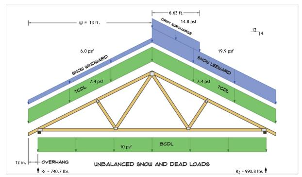
$R_1 = D + S = 431.8 \text{ lbs} + 308.9 \text{ lbs}$  $R_2 = D + S = 431.8 \text{ lbs} + 558.9 \text{ lbs}$
