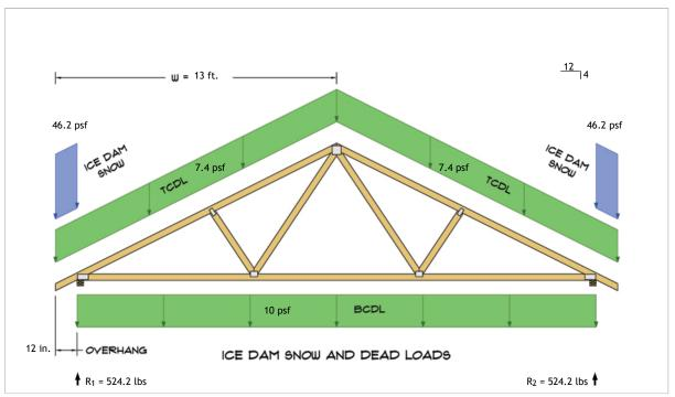
$$\begin{split} R_1 &= D + S = 431.8 \text{ lbs} + 92.4 \text{ lbs} \\ R_2 &= D + S = 431.8 \text{ lbs} + 92.4 \text{ lbs} \end{split}$$
