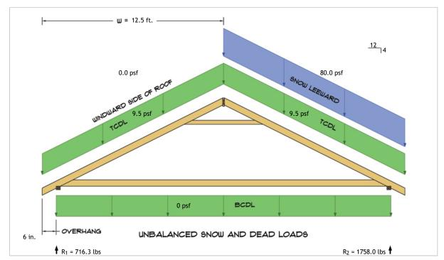
$R_1 = D + S = 237.2 \text{ lbs} + 479.2 \text{ lbs}$  $R_2 = D + S = 237.2 \text{ lbs} + 1520.8 \text{ lbs}$
