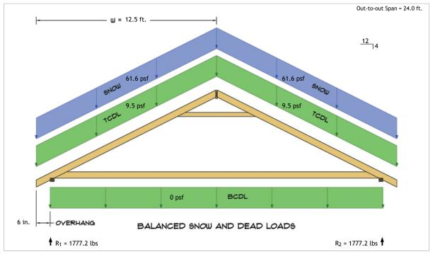
$R_1 = D + S = 237.2 \text{ lbs} + 1540.0 \text{ lbs}$  $R_2 = D + S = 237.2 \text{ lbs} + 1540.0 \text{ lbs}$
