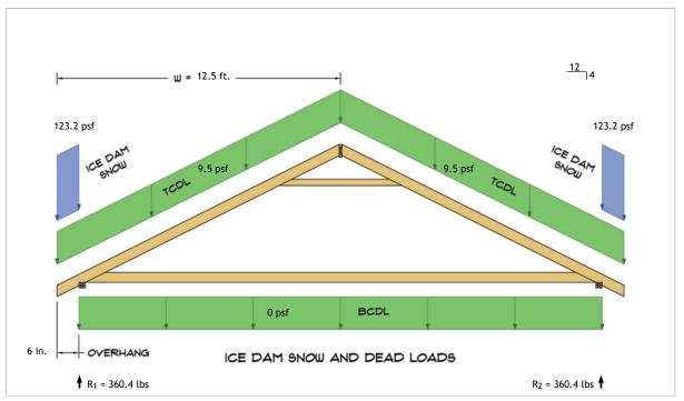
$$\begin{split} R_1 &= D + S = 237.2 \text{ lbs} + 123.2 \text{ lbs} \\ R_2 &= D + S = 237.2 \text{ lbs} + 123.2 \text{ lbs} \end{split}$$
