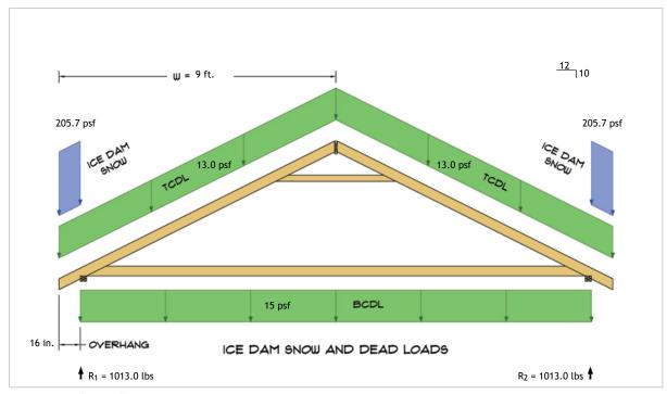
$R_1 = D + S = 464.3 \text{ lbs} + 548.7 \text{ lbs}$  $R_2 = D + S = 464.3 \text{ lbs} + 548.7 \text{ lbs}$
