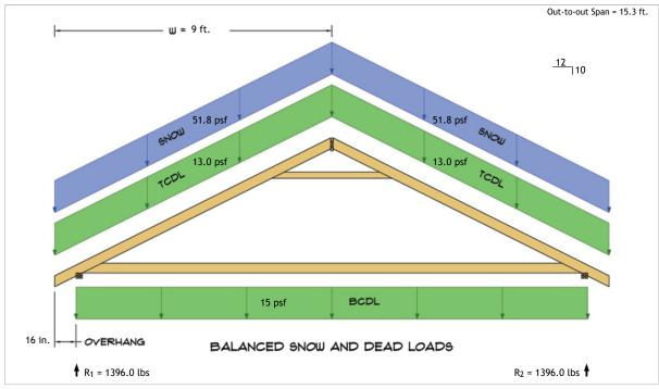
$R_1 = D + S = 464.3 \text{ lbs} + 931.7 \text{ lbs}$  $R_2 = D + S = 464.3 \text{ lbs} + 931.7 \text{ lbs}$
