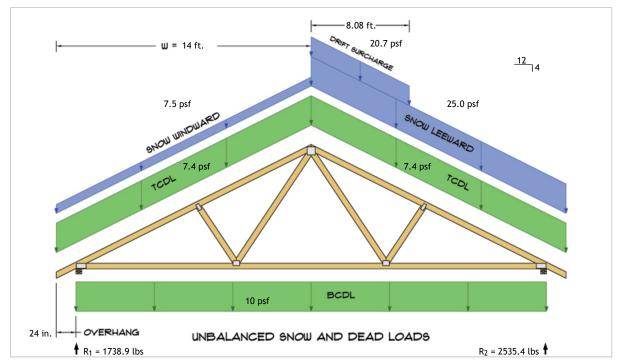
$R_1 = D + S = 893.2 \text{ lbs} + 845.7 \text{ lbs}$  $R_2 = D + S = 893.2 \text{ lbs} + 1642.2 \text{ lbs}$
