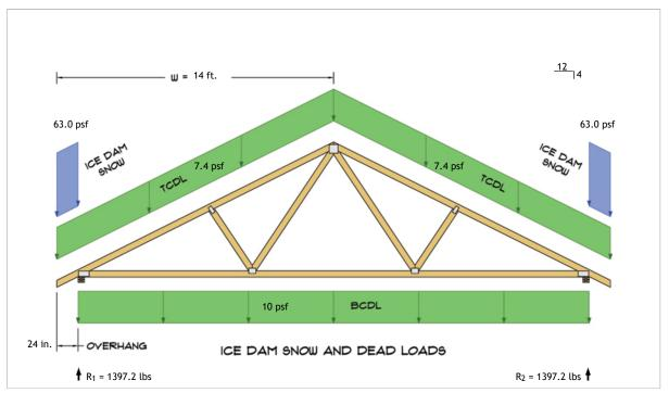
$$\begin{split} R_1 &= D + S = 893.2 \text{ lbs} + 504.0 \text{ lbs} \\ R_2 &= D + S = 893.2 \text{ lbs} + 504.0 \text{ lbs} \end{split}$$
