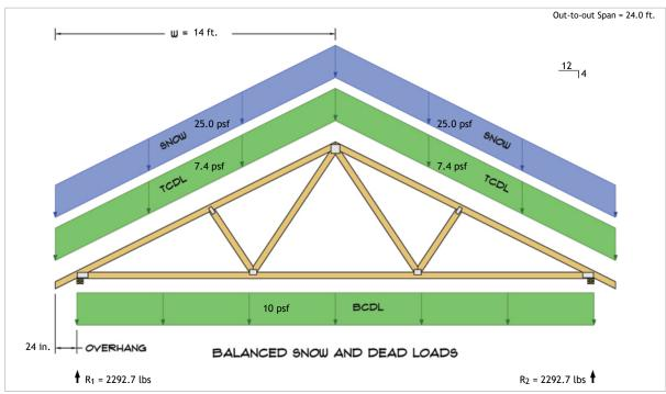
$$\begin{split} R_1 &= D + S = 893.2 \text{ lbs} + 1399.5 \text{ lbs} \\ R_2 &= D + S = 893.2 \text{ lbs} + 1399.5 \text{ lbs} \end{split}$$
