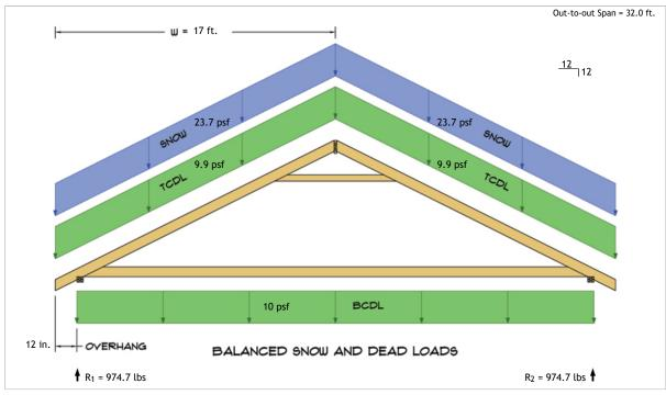
$R_1 = D + S = 437.7 \text{ lbs} + 537.0 \text{ lbs}$  $R_2 = D + S = 437.7 \text{ lbs} + 537.0 \text{ lbs}$
