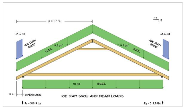
$R_1 = D + S = 437.7 \text{ lbs} + 82.1 \text{ lbs}$  $R_2 = D + S = 437.7 \text{ lbs} + 82.1 \text{ lbs}$
