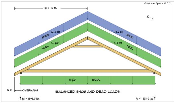
$R_1 = D + S = 499.2 \text{ lbs} + 1095.8 \text{ lbs}$  $R_2 = D + S = 499.2 \text{ lbs} + 1095.8 \text{ lbs}$
