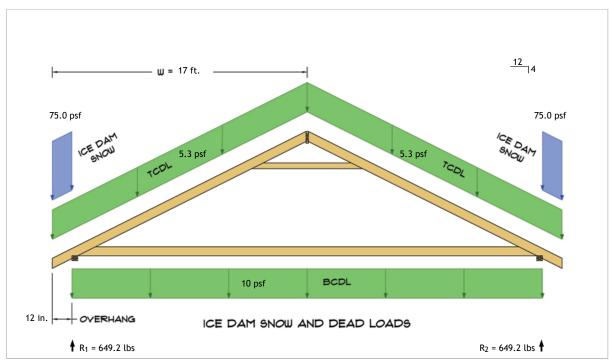
$R_1 = D + S = 499.2 \text{ lbs} + 150.0 \text{ lbs}$  $R_2 = D + S = 499.2 \text{ lbs} + 150.0 \text{ lbs}$
