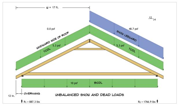
$R_1 = D + S = 499.2 \text{ lbs} + 388.1 \text{ lbs}$  $R_2 = D + S = 499.2 \text{ lbs} + 1267.7 \text{ lbs}$
