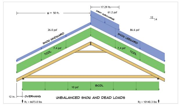
$R_1 = D + S = 1717.9 \text{ lbs} + 4955.2 \text{ lbs}$  $R_2 = D + S = 1717.9 \text{ lbs} + 8422.4 \text{ lbs}$
