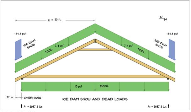
$$\begin{split} R_1 &= D + S = 1717.9 \text{ lbs} + 369.6 \text{ lbs} \\ R_2 &= D + S = 1717.9 \text{ lbs} + 369.6 \text{ lbs} \end{split}$$
