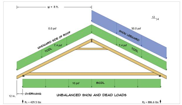
$R_1 = D + S = 258.1 \text{ lbs} + 171.4 \text{ lbs}$  $R_2 = D + S = 258.1 \text{ lbs} + 628.6 \text{ lbs}$
