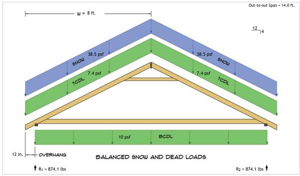
$R_1 = D + S = 258.1 \text{ lbs} + 616.0 \text{ lbs}$  $R_2 = D + S = 258.1 \text{ lbs} + 616.0 \text{ lbs}$
