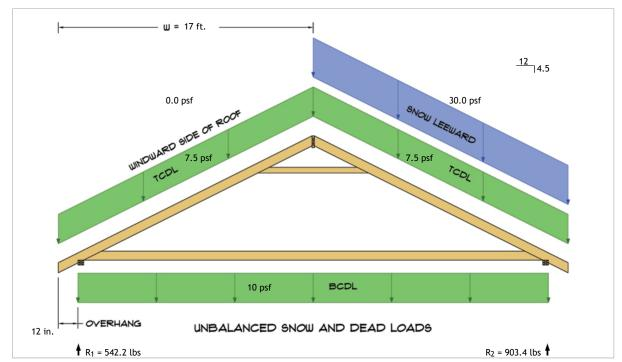
$R_1 = D + S = 382.8 \text{ lbs} + 159.4 \text{ lbs}$  $R_2 = D + S = 382.8 \text{ lbs} + 520.6 \text{ lbs}$
