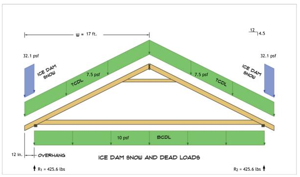
$$\begin{split} R_1 &= D + S = 382.8 \text{ lbs} + 42.8 \text{ lbs} \\ R_2 &= D + S = 382.8 \text{ lbs} + 42.8 \text{ lbs} \end{split}$$
