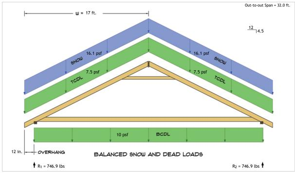
$R_1 = D + S = 382.8 \text{ lbs} + 364.1 \text{ lbs}$  $R_2 = D + S = 382.8 \text{ lbs} + 364.1 \text{ lbs}$
