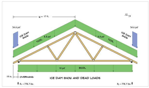
$\begin{aligned} R_1 &= D + S = 605.8 \text{ lbs} + 172.9 \text{ lbs} \\ R_2 &= D + S = 605.8 \text{ lbs} + 172.9 \text{ lbs} \end{aligned}$
