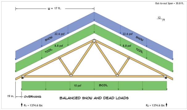
$R_1 = D + S = 605.8 \text{ lbs} + 768.8 \text{ lbs}$  $R_2 = D + S = 605.8 \text{ lbs} + 768.8 \text{ lbs}$
