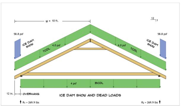
$R_1 = D + S = 152.3 \text{ lbs} + 117.6 \text{ lbs}$  $R_2 = D + S = 152.3 \text{ lbs} + 117.6 \text{ lbs}$
