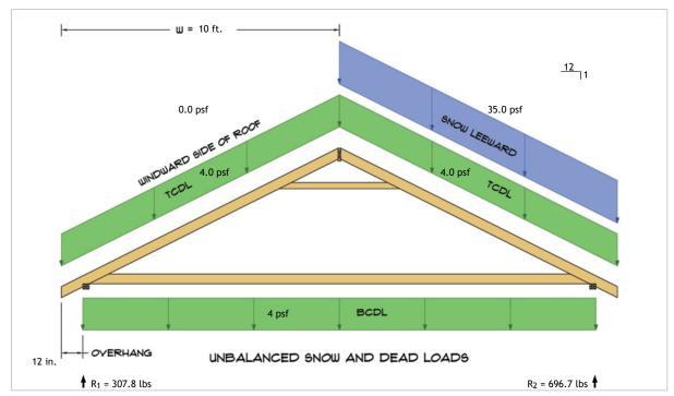
$R_1 = D + S = 152.3 \text{ lbs} + 155.6 \text{ lbs}$  $R_2 = D + S = 152.3 \text{ lbs} + 544.4 \text{ lbs}$
