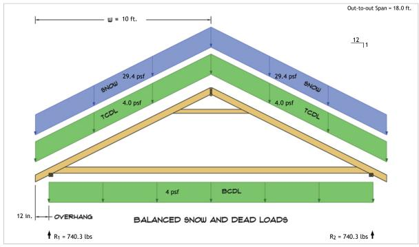
$R_1 = D + S = 152.3 \text{ lbs} + 588.0 \text{ lbs}$  $R_2 = D + S = 152.3 \text{ lbs} + 588.0 \text{ lbs}$
