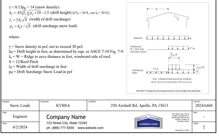
For a roof rafter system with  $W \le 20$  ft., the simplified unbalanced snow load is given by the third diagram of ASCE Figure 7-5.
