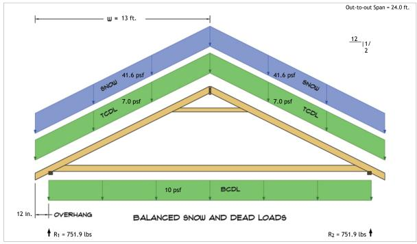
$R_1 = D + S = 211.3 \text{ lbs} + 540.5 \text{ lbs}$  $R_2 = D + S = 211.3 \text{ lbs} + 540.5 \text{ lbs}$
