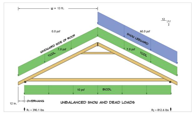
$R_1 = D + S = 211.3 \text{ lbs} + 178.8 \text{ lbs}$  $R_2 = D + S = 211.3 \text{ lbs} + 601.3 \text{ lbs}$
