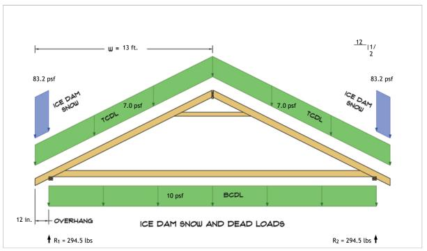
$$\begin{split} R_1 &= D + S = 211.3 \text{ lbs} + 83.2 \text{ lbs} \\ R_2 &= D + S = 211.3 \text{ lbs} + 83.2 \text{ lbs} \end{split}$$
