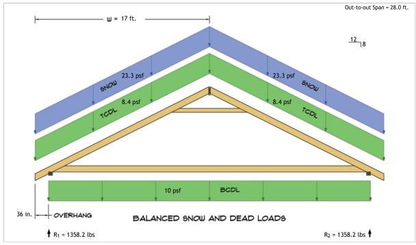
$R_1 = D + S = 566.0 \text{ lbs} + 792.2 \text{ lbs}$  $R_2 = D + S = 566.0 \text{ lbs} + 792.2 \text{ lbs}$
