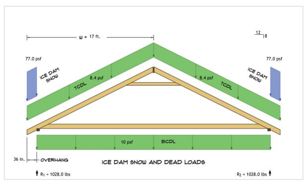
$R_1 = D + S = 566.0 \text{ lbs} + 462.0 \text{ lbs}$  $R_2 = D + S = 566.0 \text{ lbs} + 462.0 \text{ lbs}$
