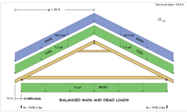
$\begin{aligned} R_1 &= D + S = 875.2 \text{ lbs} + 8320.1 \text{ lbs} \\ R_2 &= D + S = 875.2 \text{ lbs} + 8320.1 \text{ lbs} \end{aligned}$
