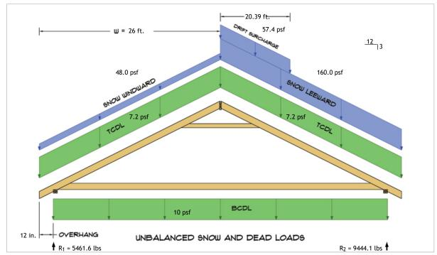
$R_1 = D + S = 875.2 \text{ lbs} + 4586.4 \text{ lbs}$  $R_2 = D + S = 875.2 \text{ lbs} + 8568.9 \text{ lbs}$
