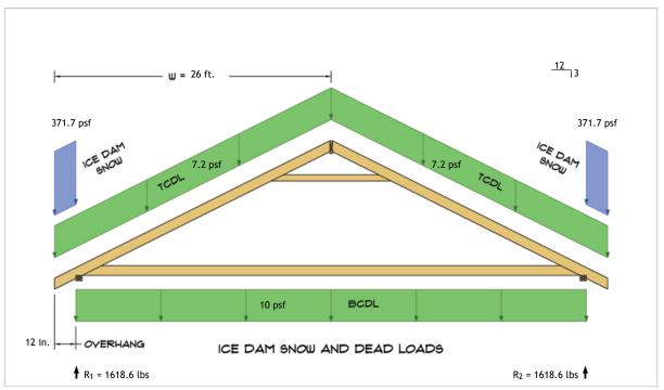
$$\begin{split} R_1 &= D + S = 875.2 \text{ lbs} + 743.4 \text{ lbs} \\ R_2 &= D + S = 875.2 \text{ lbs} + 743.4 \text{ lbs} \end{split}$$
