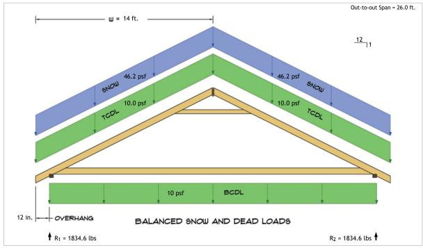
$R_1 = D + S = 541.0 \text{ lbs} + 1293.6 \text{ lbs}$  $R_2 = D + S = 541.0 \text{ lbs} + 1293.6 \text{ lbs}$
