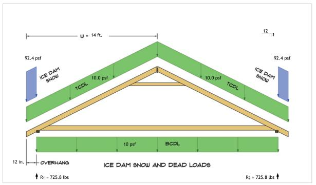
$$\begin{split} R_1 &= D + S = 541.0 \text{ lbs} + 184.8 \text{ lbs} \\ R_2 &= D + S = 541.0 \text{ lbs} + 184.8 \text{ lbs} \end{split}$$
