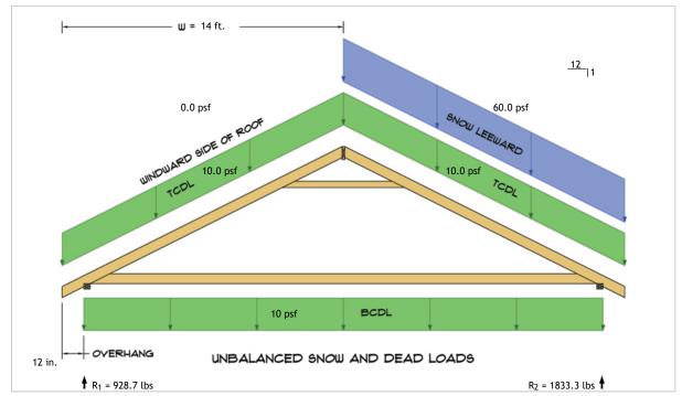
$R_1 = D + S = 541.0 \text{ lbs} + 387.7 \text{ lbs}$  $R_2 = D + S = 541.0 \text{ lbs} + 1292.3 \text{ lbs}$
