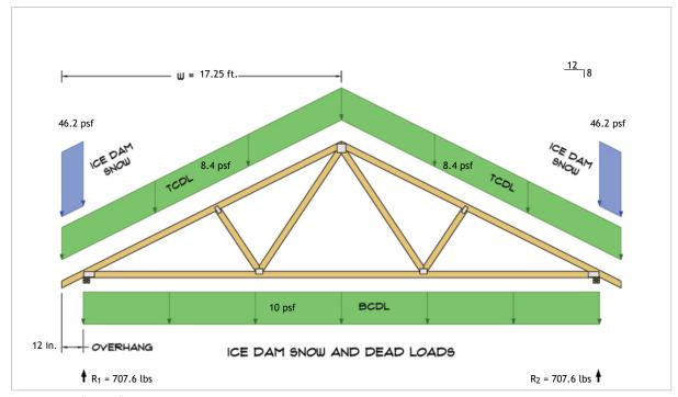
$R_1 = D + S = 615.2 \text{ lbs} + 92.4 \text{ lbs} \\ R_2 = D + S = 615.2 \text{ lbs} + 92.4 \text{ lbs}$
