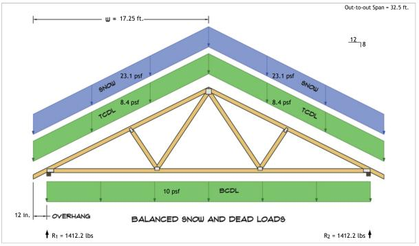
$R_1 = D + S = 615.2 \text{ lbs} + 797.0 \text{ lbs}$  $R_2 = D + S = 615.2 \text{ lbs} + 797.0 \text{ lbs}$
