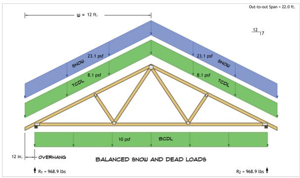
$$\begin{split} R_1 &= D + S = 414.5 \text{ lbs} + 554.4 \text{ lbs} \\ R_2 &= D + S = 414.5 \text{ lbs} + 554.4 \text{ lbs} \end{split}$$
