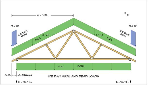
$$\begin{split} R_1 &= D + S = 414.5 \text{ lbs} + 92.4 \text{ lbs} \\ R_2 &= D + S = 414.5 \text{ lbs} + 92.4 \text{ lbs} \end{split}$$
