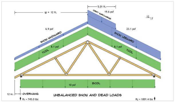
$R_1 = D + S = 414.5 \text{ lbs} + 330.5 \text{ lbs}$  $R_2 = D + S = 414.5 \text{ lbs} + 586.9 \text{ lbs}$
