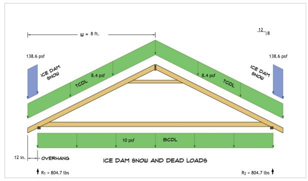
$\begin{aligned} R_1 &= D + S = 400.5 \text{ lbs} + 404.3 \text{ lbs} \\ R_2 &= D + S = 400.5 \text{ lbs} + 404.3 \text{ lbs} \end{aligned}$
