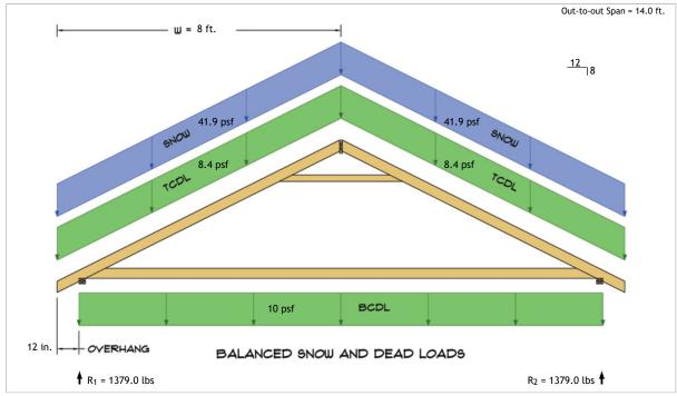
$R_1 = D + S = 400.5 \text{ lbs} + 978.6 \text{ lbs}$  $R_2 = D + S = 400.5 \text{ lbs} + 978.6 \text{ lbs}$
