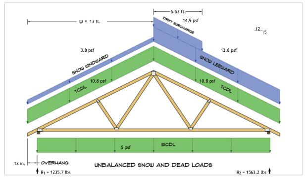
$R_1 = D + S = 803.3 \text{ lbs} + 432.3 \text{ lbs}$  $R_2 = D + S = 803.3 \text{ lbs} + 759.9 \text{ lbs}$
