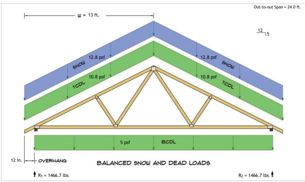
$$\begin{split} R_1 &= D + S = 803.3 \text{ lbs} + 663.3 \text{ lbs} \\ R_2 &= D + S = 803.3 \text{ lbs} + 663.3 \text{ lbs} \end{split}$$
