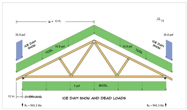
$$\begin{split} R_1 &= D + S = 803.3 \text{ lbs} + 140.0 \text{ lbs} \\ R_2 &= D + S = 803.3 \text{ lbs} + 140.0 \text{ lbs} \end{split}$$
