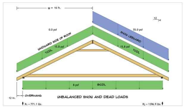
$R_1 = D + S = 497.3 \text{ lbs} + 273.8 \text{ lbs}$  $R_2 = D + S = 497.3 \text{ lbs} + 899.6 \text{ lbs}$
