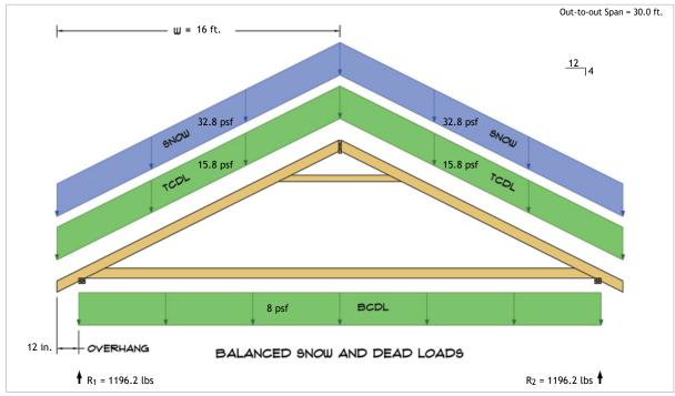
$R_1 = D + S = 497.3 \text{ lbs} + 698.9 \text{ lbs}$  $R_2 = D + S = 497.3 \text{ lbs} + 698.9 \text{ lbs}$
