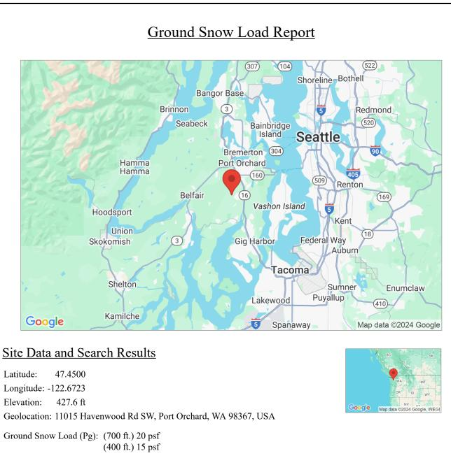
\*Numbers in parenthesis represent the upper elevation limits in feet for the ground snow loads presented.
