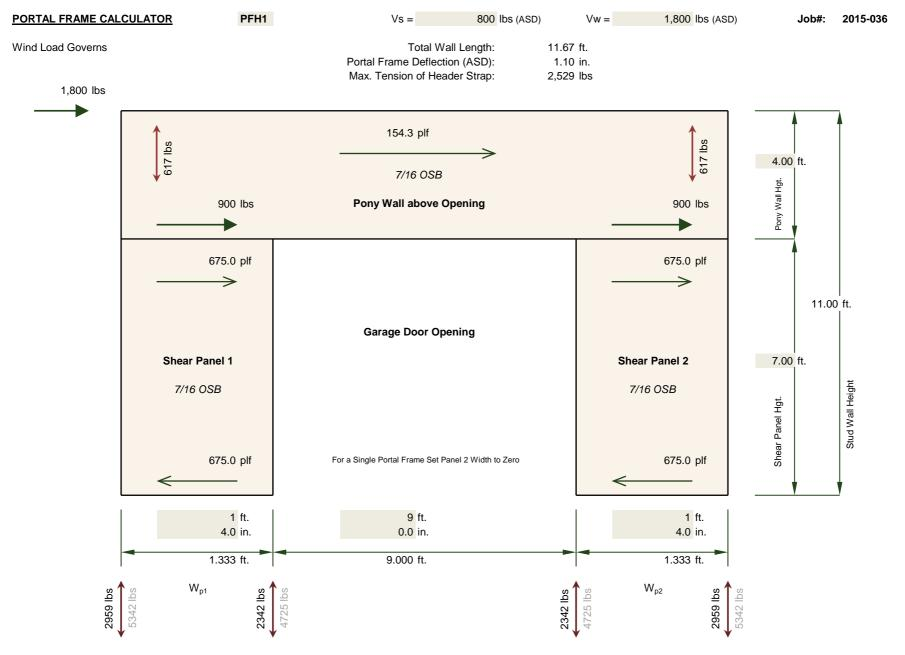
\*Notes: 1.) Shear Distribution based on equivalent deflection of each shear panel.
