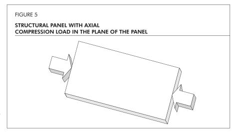
ity is given as F<sub>c</sub>A, where F<sub>c</sub> is the allowable axial compression stress of the material, and A is the area of the cross section. Units of F<sub>c</sub>A are lbf per foot of panel width. Axial compression strength is illustrated in Figure 5.
