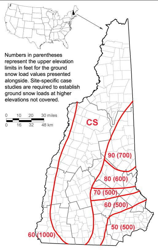
Figure 1. State of New Hampshire, showing town and county boundaries overlaid with the ground snow load information in ASCE 7. (To convert  $lb/ft^2$  to  $kN/m^2$ , multiply by 0.048; for ft to m, multiply by 0.305.)
