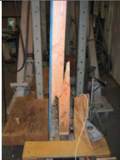
Figure B7. End post failure of Wall 2.
