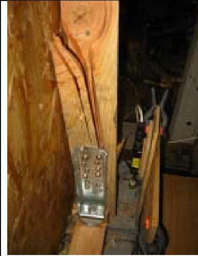
Figure B7. End post failure of Wall 2.
