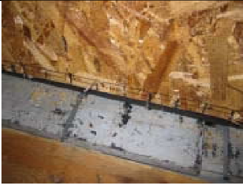
Figure B3. Typical nail yield and subsequent withdrawal from sill plate. Wall 5.
