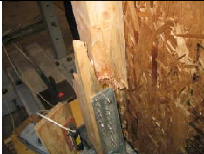
Figure B8. End post failure of Wall 2.
