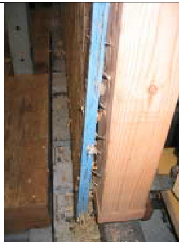
Figure B4. Nail withdrawn after testing. Typical nail yielding controlling shear wall failure. Wall 5.
