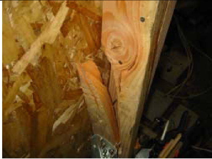
Figure B8. End post failure of Wall 2.
