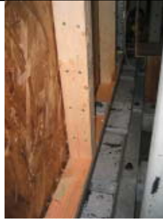
Figure B2. Stitch nailed double 2x in Wall 8. Photo was taken after testing was complete. Note: OSB panel separation from framing at sill plate, also parallel line marks on double 2x for visual observation during testing.
